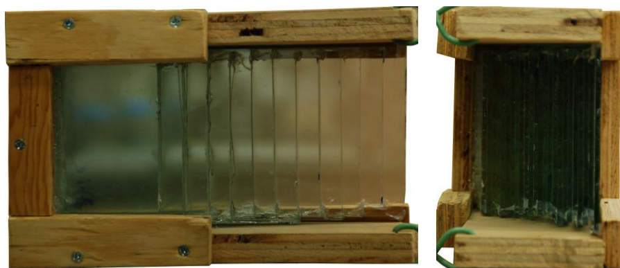
Figure 3.15: Images of the glass plate wedge used to find beam hardening parameter for the glass bead bed.
